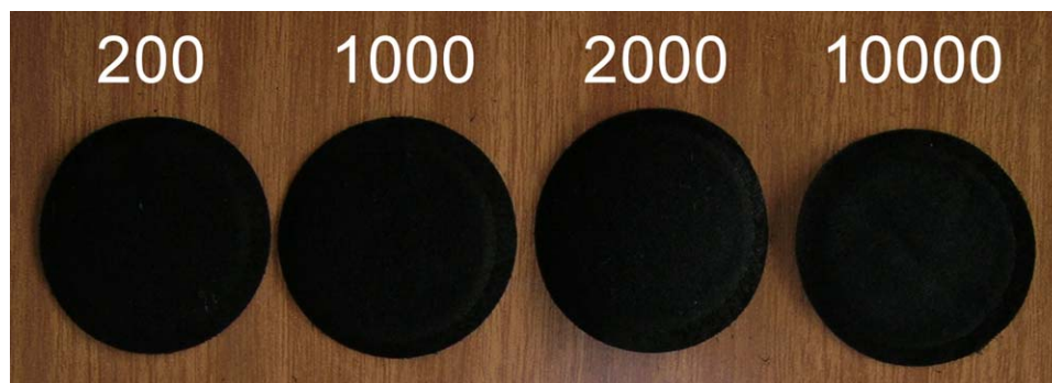
Figure 4. Picture of the specimens after abrasion tests (200, 1000, 2000, and 10,000 abrasion cycles). [Color figure can be viewed in the online issue, which is available at wileyonlinelibrary.com .]
